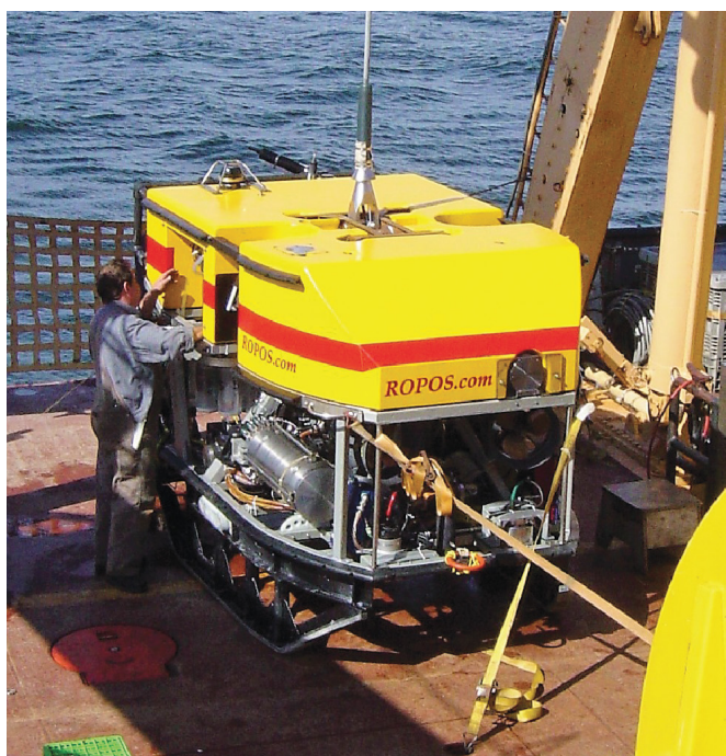
Fig 3 The Remotely Operate Vehicle for Ocean Sciences (ROPOS) is deployed from a surface ship on a fibre optic tether that allows scientists to watch real time video feed on board the ship and even from land via satellite relay. Manipulator arms are used to collect samples and facilitate measurements. Photo courtesy of PVRs.
